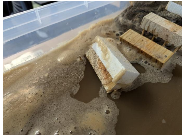
Figure 13: The amphibious houses rose with the water as expected, but they also introduced an unexpected mode of failure, in which a house flipped upside down after rising above its guideposts.
