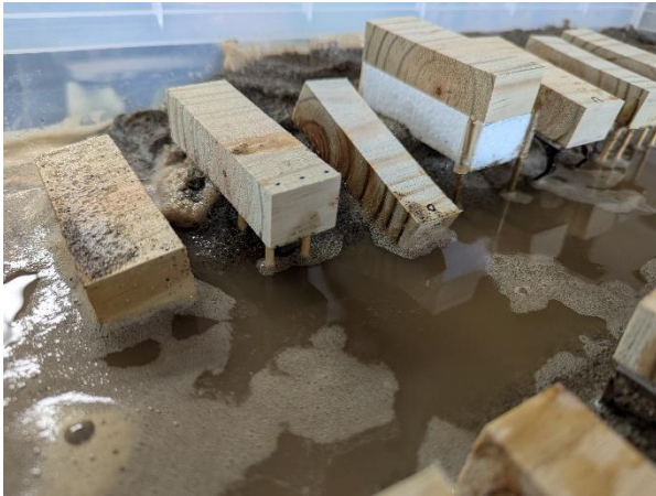
Figure 10: The first building to fail was a control house that had no foundation at all.
