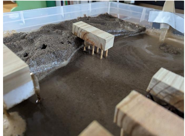
Figure 12: All houses on medium and deep piles remained standing, even after a substantial amount of sand had washed away from underneath them. This indicated that excessively deep piles would not provide proportional performance benefits within this context, reinforcing the value of moderate elevation strategies.
