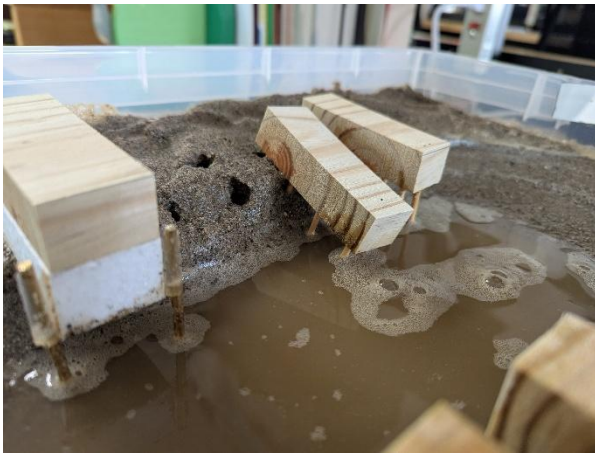
Figure 11: The second building to fail was a house on short foundation piles.
